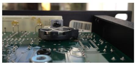
The following shows the soldering of the new battery holder seen from the top of the circuit board with the minus pole pin soldered to the same solder joint as previously the old battery's negative pole was soldered and the plus pole pin of the holder soldered to the frontmost of the two solder joints:
