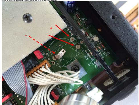
The circle corresponds roughly to the size of the old battery. To the left is the prong (minus pole, broken red arrow) having been attached to the old battery's bottom. This prong's pin is still soldered to the circuit board. The larger prong (positive pole, two red arrows) had 2 pins (now empty holes to the right of the circle) and was soldered to the top of the old battery. This design is awful and it is very cumbersome to replace a battery. I decided to change that.
